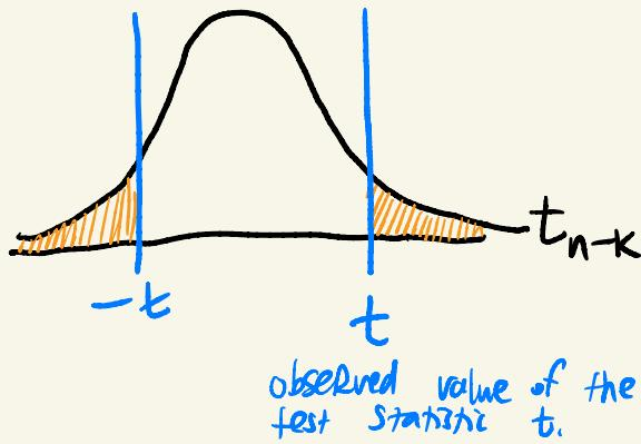
The **p-value** is the orange area to the Right of  $t$  and left of  $-t$  Under the  $t_{n-k}$  density curve. It is, assuming the null  $H_0$  is true, the probability of observing a test statistic as extreme as the one we actually observed, where the randomness here is over the sampling distribution (generating  $y$  from  $x$ ).
